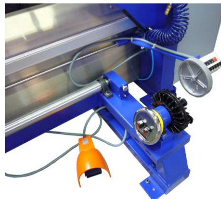
Click-bearings with brake, meter counter and foot-pedal
